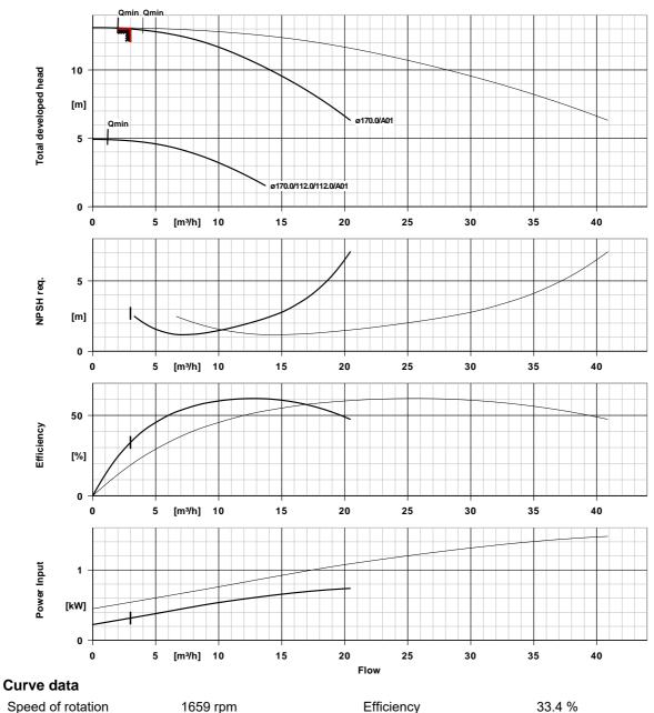
Speed of rotation1659 rpmFluid density999 kg/m³Viscosity1.25 mm²/sFlow rate3.00 m³/hRequested flow rate3.00 m³/hTotal developed head13.00 mRequested developed head13.00 m
