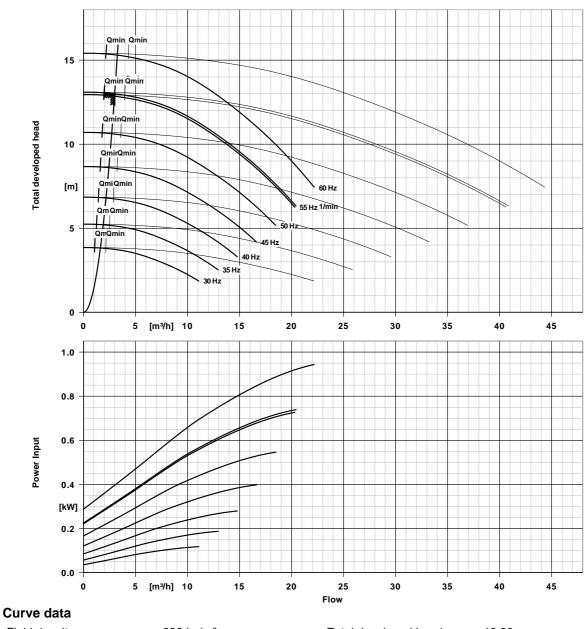
Fluid density Viscosity Flow rate Requested flow rate 999 kg/m<sup>3</sup> 1.25 mm<sup>2</sup>/s 3.00 m<sup>3</sup>/h 3.00 m<sup>3</sup>/h Total developed head13.00 mRequested developed head13.00 mMEI (Minimum Efficiency $\geq 0.70$ Index)Effective impeller diameter170.0 mm
