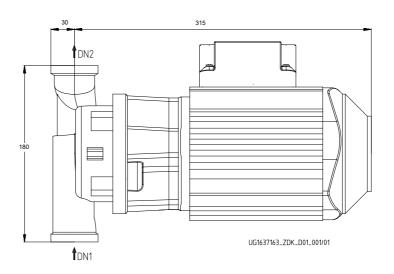
Drawing is not to scale Dimensions in mm
