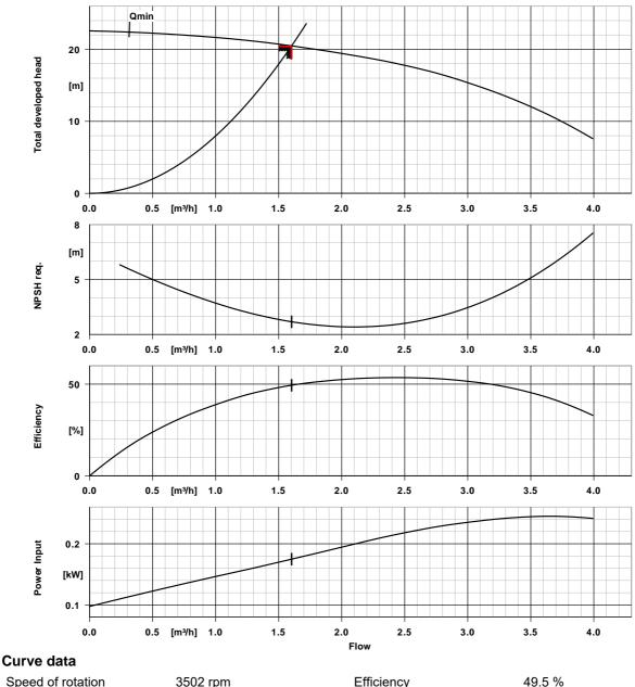
Speed of rotation3502 rpmFluid density965 kg/m³Viscosity0.33 mm²/sFlow rate1.60 m³/hRequested flow rate1.60 m³/hTotal developed head20.49 mRequested developed head20.41 m
